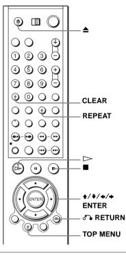
Press  $\triangleq$  and place a DATA CD on the disc tray, then press  $\triangleq$  to close the tray.
